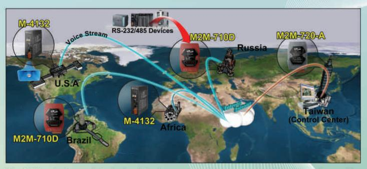
The M2M series is specially designed for the remote maintenance and serial to network upgrading solution. This module provides 2 major technologies on networking: Voice streaming and Pair connection. The Pair connection provides TCP data tunneling between 2 serial devices so that the user can operate remote COM port device via Ethernet TCP/IP protocol just like a local COM port. The Voice streaming allows user to talk to remote operator while operate remote COM-linked devices.
