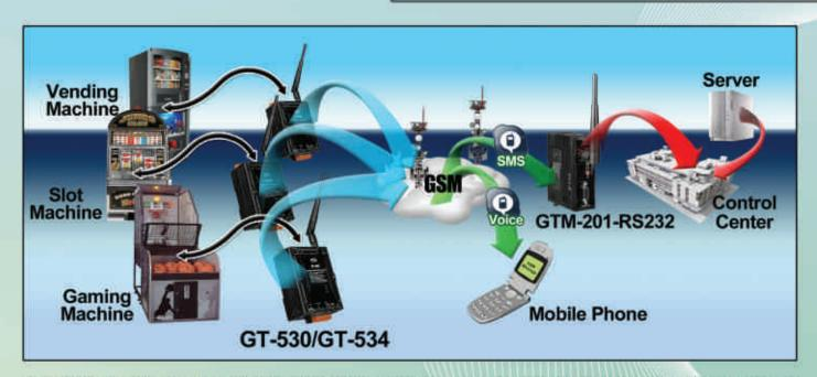
ICP DAS provides various intelligent 2G/3G modules and gateway, GT-5xx Series. The module is GSM remote control and alarm system allows users to use their mobile phone to monitor and control the business from any location. Its alarm facilities provide a flexible way to distribute critical alarm information to any number of mobile phone users. The Gateway allows user to access mobile phone by using standard protocol, such as Modbus.
