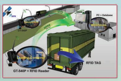
ICP DAS provides SST series which is designed for data acquisition and control applications between a host and remote sensors. It is also useful for those applications where the installation of cable wire is inconvenient. The SST Series is a spread spectrum radio modem with an RS-232/RS-485 interface port.
