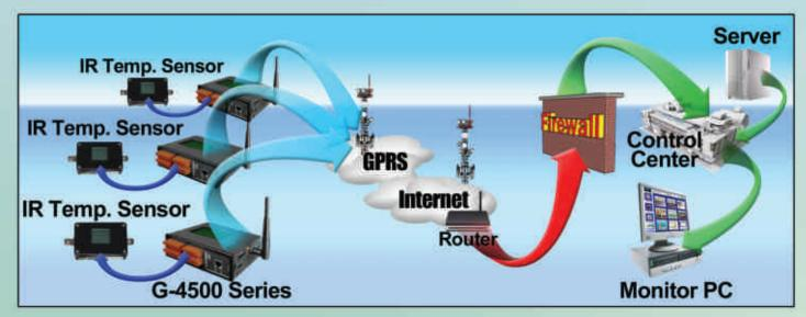
The G-4500 series provided by ICP DAS are M2M mini programmable automation controller with a cellular transceiver can monitor industrial equipment that sends live data to the monitoring system, providing real-time status. With optional GPS model, the G-4500 can also be a GPS tracking system. It can be used in vehicle management or maritime system.
